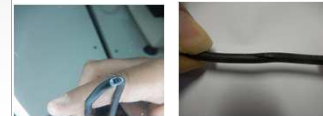
Dielectric test with puncturing of the sample 17 under 1,2 kVab when should withstand until 3,5 kVab/5 min Cable 5,2 mm2 - EPR ; Use: slip ring of generator
