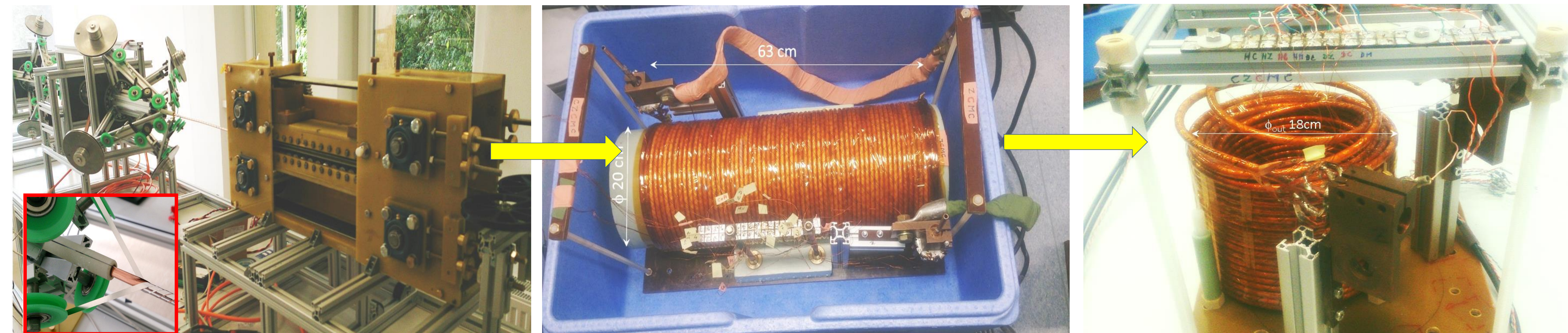
Cabling machine and detail showing the tape depositing on cable core
